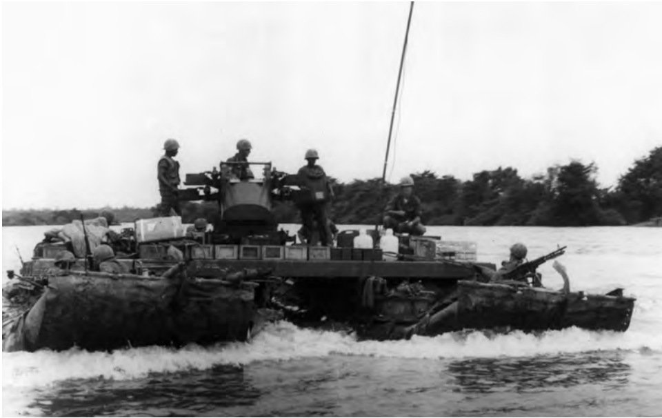
Men of the 1st Engineer Battalion use an M4T6 raft as a patrol boat.
